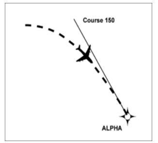
(4) Radius to Fix. A Radius to Fix (RF) leg is defined as a constant radius circular path around a defined turn center that terminates at a fix. See FIG 1–2–6.
