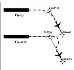
FIG 1-2-2 Fly-by and Fly-over Waypoints
