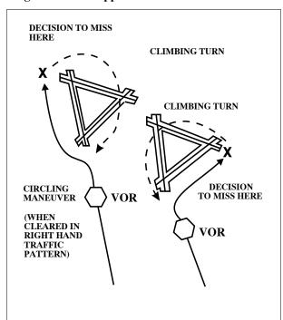
FIG 5-4-30 Circling and Missed Approach Obstruction Clearance Areas
