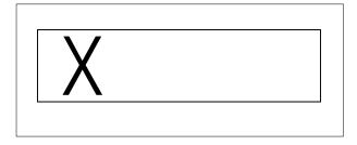
**d.** Marking and Lighting of Permanently Closed Runways and Taxiways. For runways and taxiways which are permanently closed, the lighting circuits will be disconnected. The runway threshold, runway designation, and touchdown markings are obliterated and yellow crosses are placed at each end of the runway and at 1,000 foot intervals. (See FIG 2–3–22.)
