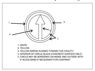
FIG 2-3-21 Nonmovement Area Boundary Markings
