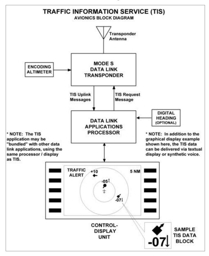
2. The cockpit equipment functionality required by a TIS client aircraft to receive the service consists of the following (refer to FIG 4-5-7):
