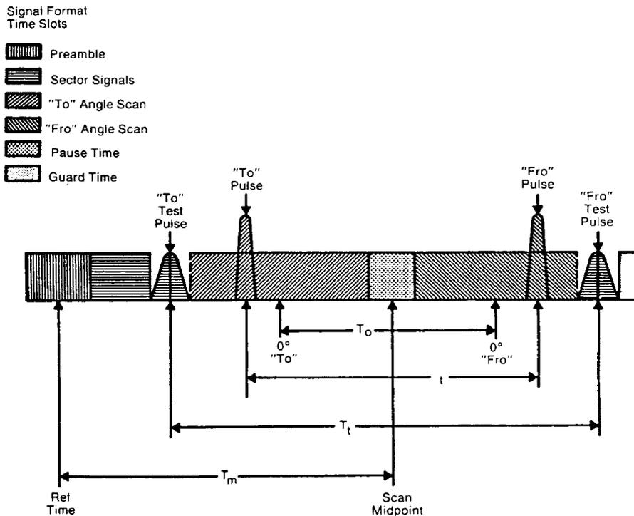
Figure 7. Azimuth Angle Scan Timing (Not to Scale)
